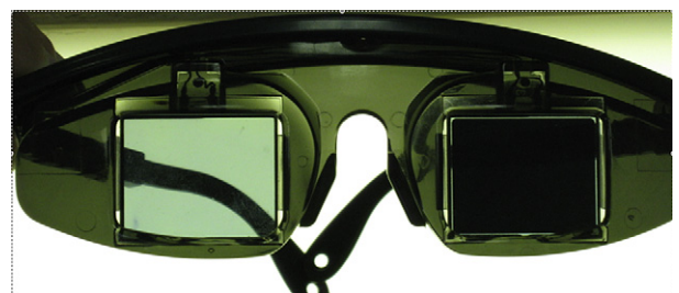
Figure 1 The alternate occlusion goggles show 1 liquid crystal lens occluded.
